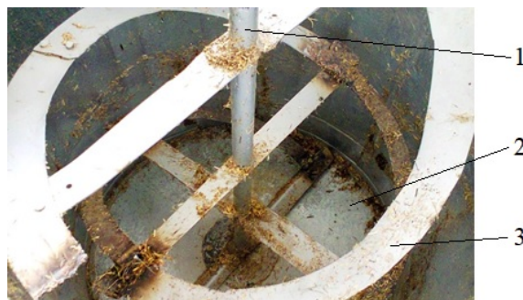
Fig. 1. Working chamber of laboratory feed mixer: 1 – shaft; 2 – working chamber bottom; 3 – tape of the helix working body
